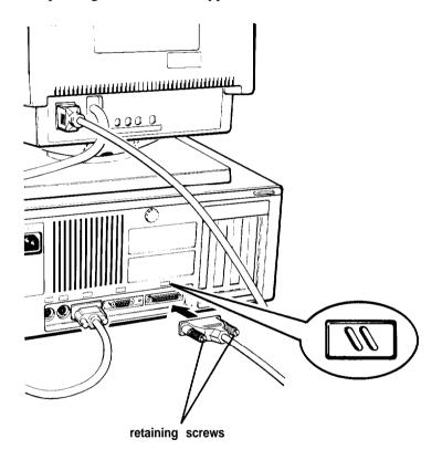
3. Connect the other end of the cable to the printer as shown below. To secure the cable, squeeze the clips at each side of the printer port and push them into place,
